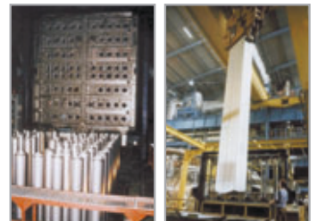
Left Piston rod with Ceraplate coating
