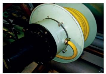
The cable drum serves as supply of electrical power and control signals to the extinguishing monitor for electrical operation by remote control. It is supplied laterally mounted to the fire fighting cylinder. The special cable is wound tightly by a spring device onto the drum and fed through the cable feed tube to a terminal block underneath the extinguishing monitor.
