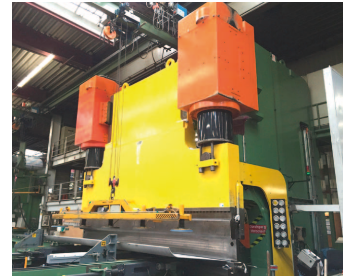
3000 ton bending press with two cylinders with Ceraplate rod coating
