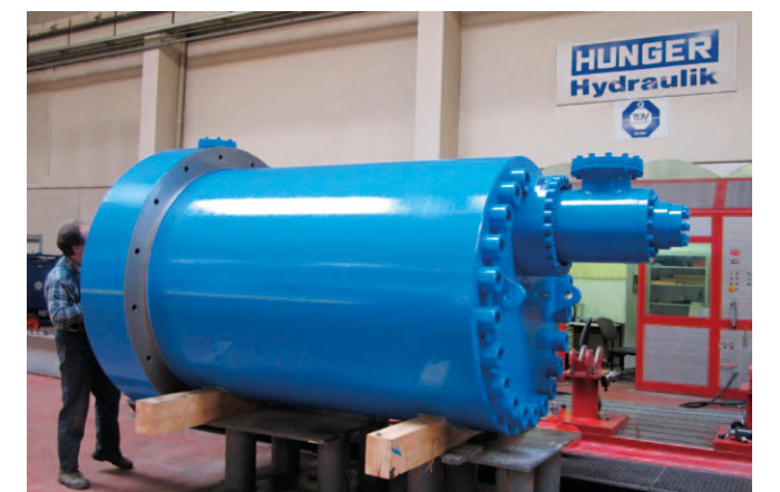
3500 ton press cylinder with mounted pre-fill valve
