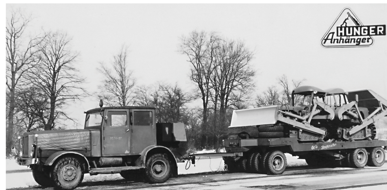
60 ton flat bed trailer with levelling hydraulic
