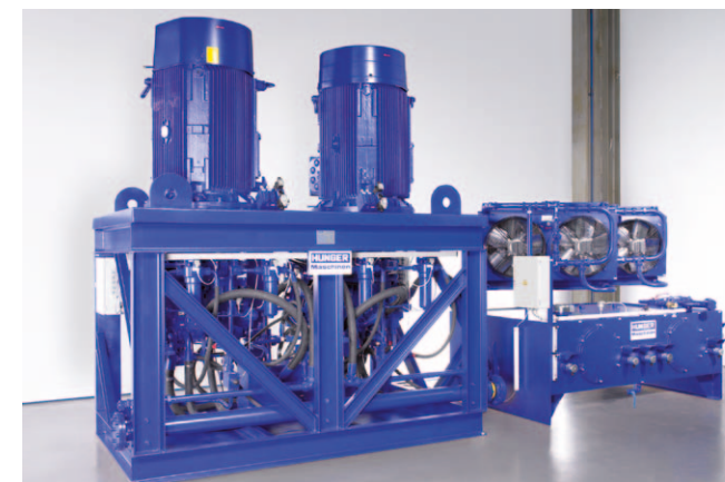
Hydraulic power unit for conveyor drive of a mobile crusher
