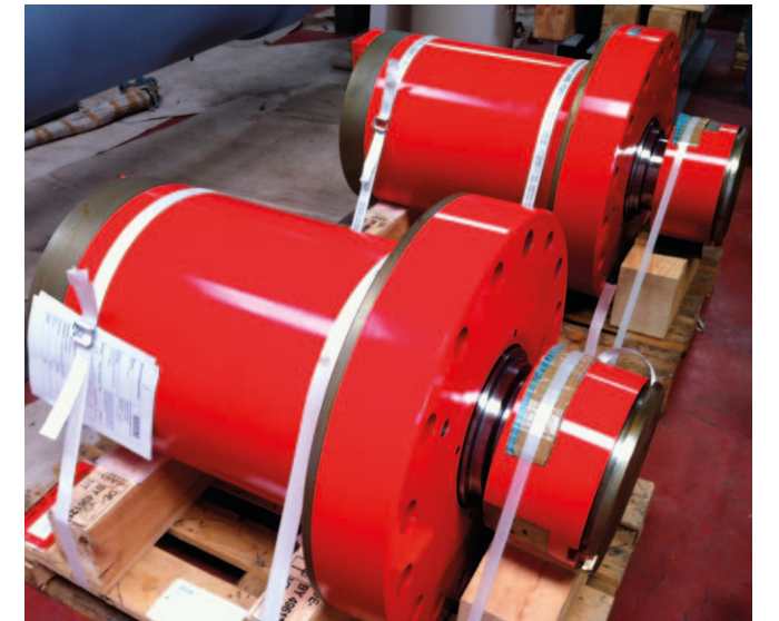
Jacking cylinder for NBR-Offshore crawler
