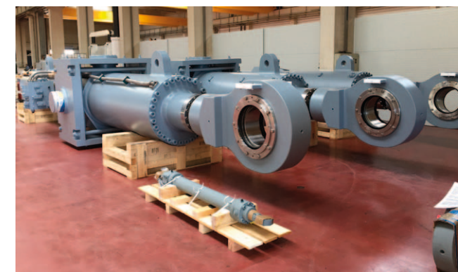
Cylinders for Boston-Barrier project / GB with immersible sectional gate
