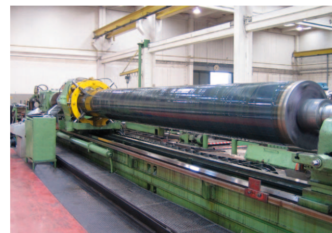
Horizontal and vertical outside and inside honing machines for surface machining of piston rods and cylinder bore holes as well as for coated surfaces
