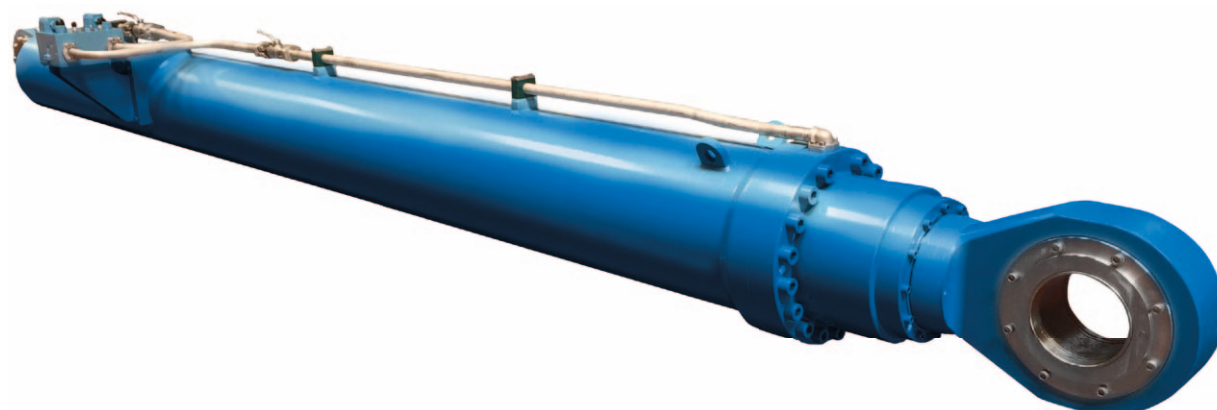
Boom cylinder for ship unloader with Ceraplate rod coating and maintenance free spherical bearings in stainless steel
