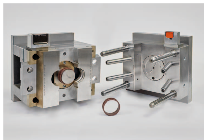
split mould for demounting more complex shaped parts, e. g. wear bands
