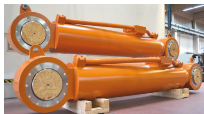
Bucket hydraulic cylinders with CeraplatePlus and CIPS
