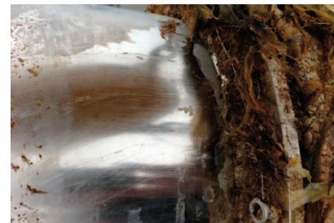
Maritime vegetal cover on a cylinder head
