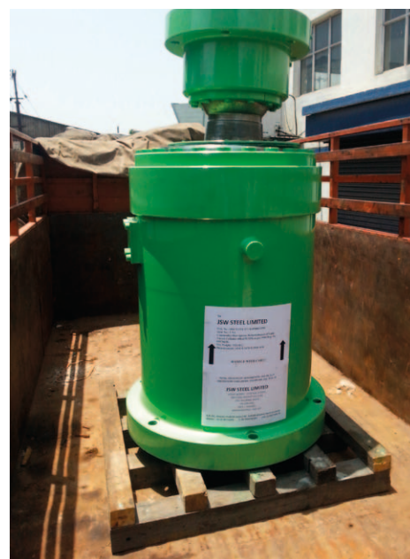
Fully overhauled ladle turret cylinder
