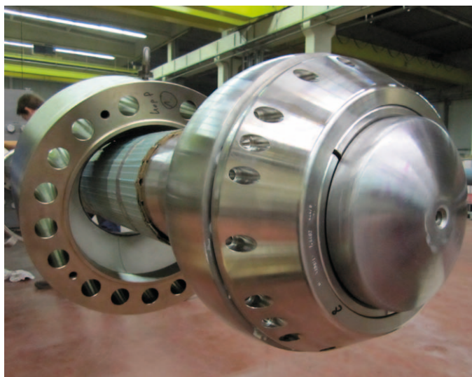
Ball joint for riser-tensioner cylinders (offshore drilling systems)
