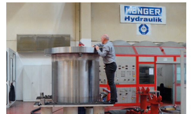
Rotary crusher cylinder on the test rig
