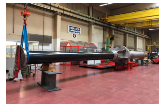
Vertical casting cylinder under works test
