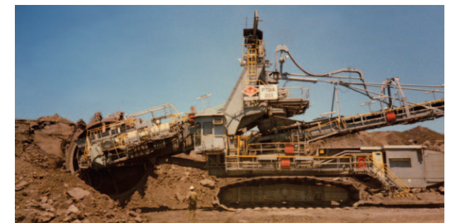
Bucket-wheel excavator with cylinders for boom and conveyor belt operation
