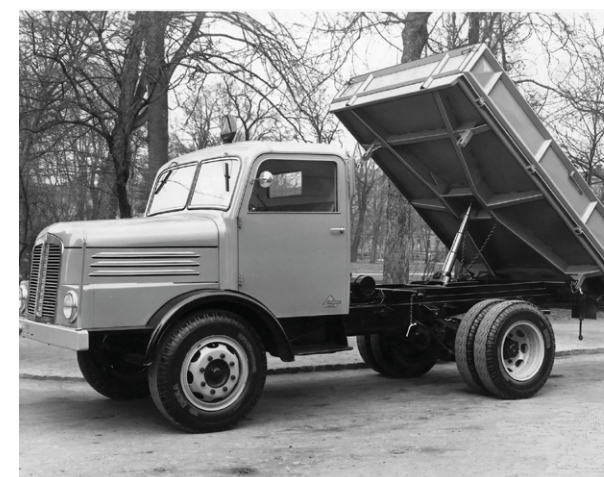
Tipper truck with telescopic cylinder
