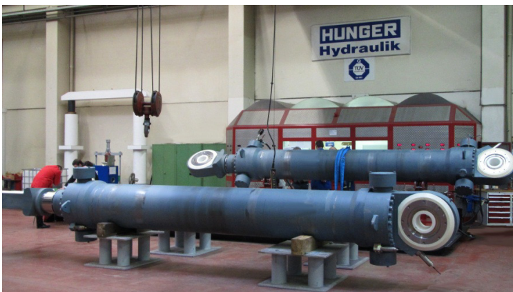
Figure 7: Oyster 800 cylinders on the hydraulic test rig
