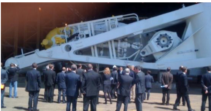
Figure 4: The cylinder module within Oyster 800
