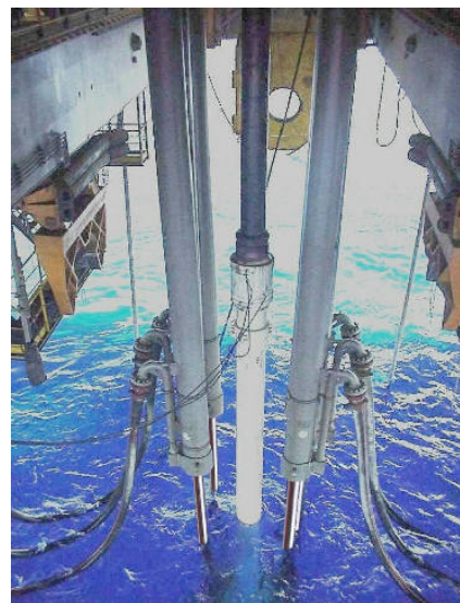
Central drill pipe supported with N-line tensioner cylinders
